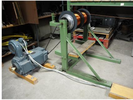
Fig. 13. Wire feeding with tension control by current-controlled DC-machine and chain drive ( $i \approx 2.2$ )
