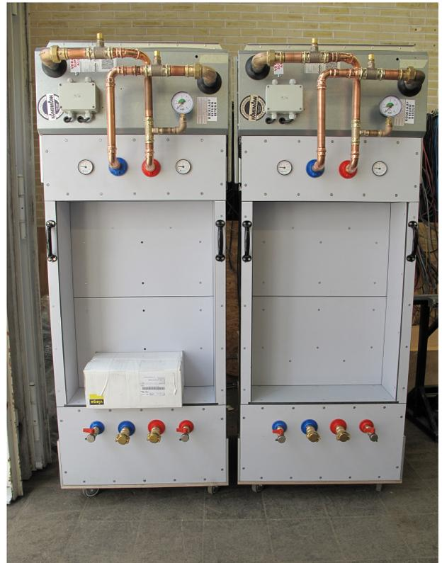
Fig. 26. Two water-to-air heat exchanger for prototype and load machine
