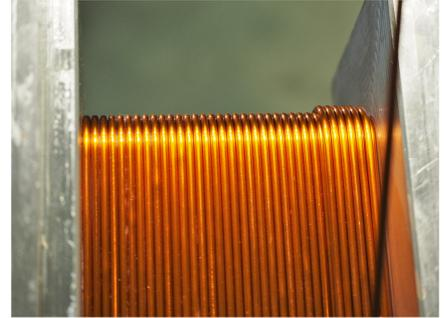
Fig. 17. Second layer orthocyclic wound (for demonstration purposes the resin is omitted)
