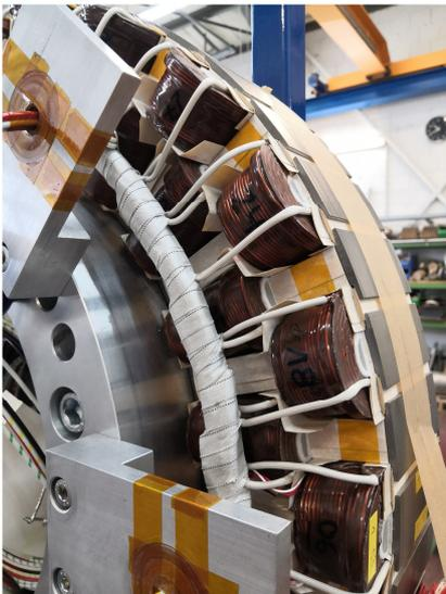
Fig. 8 Stator interconnection prior to impregnation, both carried out by *Brenner [ii]*
