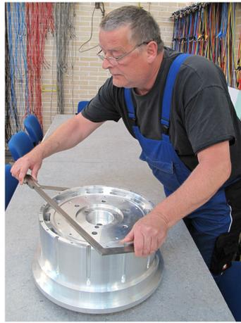
Fig. 3 Stator support after machining.
