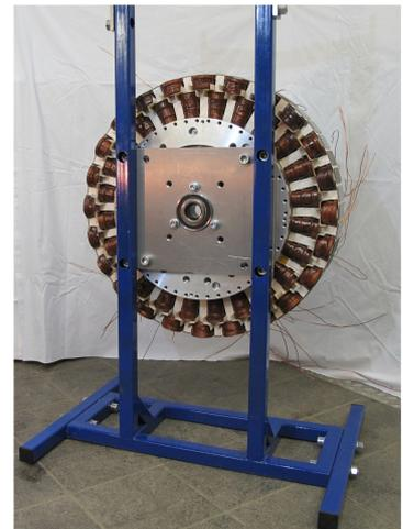
Fig. 7 Assembled stator prior to interconnection and impregnation on mounting support (blue)
