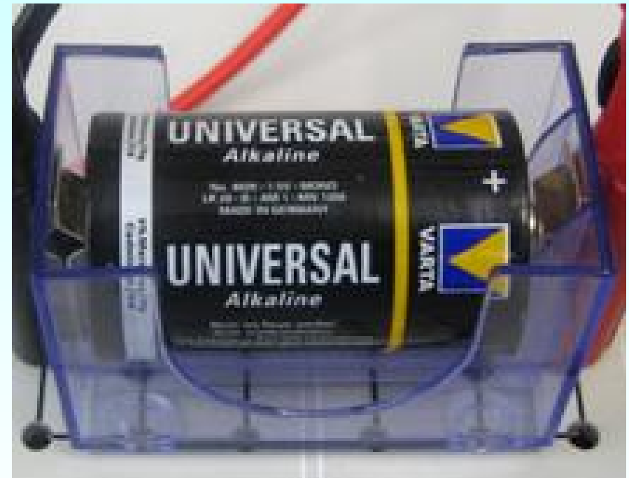
Alkali-Zink-Element (1.5 V = 1 Zelle)
