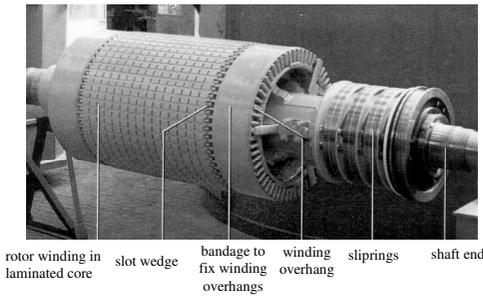
Fig. 5.19: Slipring rotor: rotor winding in laminated core, right: sliprings
