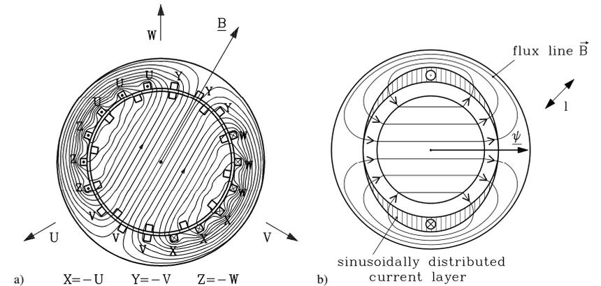
Fig. 5.2: Two-pole slipring induction motor, supplied with three-phase current, rotor at zero current:
