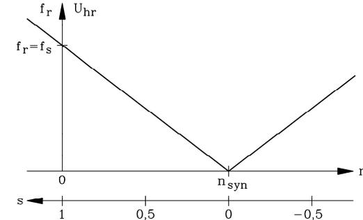
Fig. 5.4: Reduction of the rotor frequency  $f_r$  with increasing speed  $n$  up to synchronous speed
