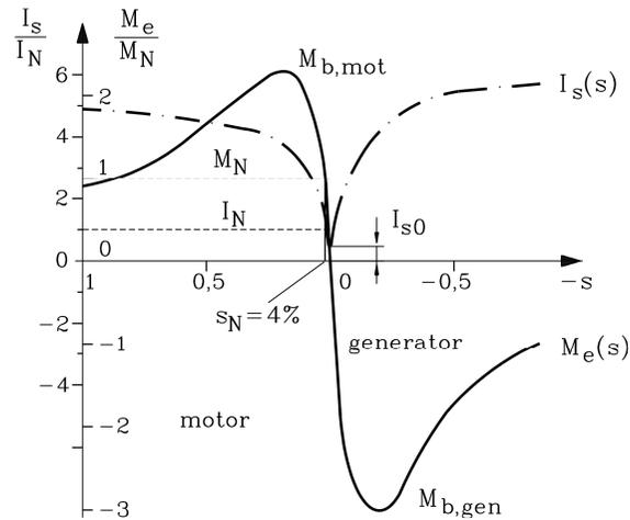
Fig. 5.8: Torque  $M_e$  and stator current  $I_s$  as functions of the slip  $s$  ( $R_s/X_s = 1/100$ ,  $R_r/X_r = 1.3/100$ ,  $\sigma = 0.067$ ,  $X_s = X_r' = 3Z_N$ ,  $Z_N = U_N/I_N$  (phase values))
