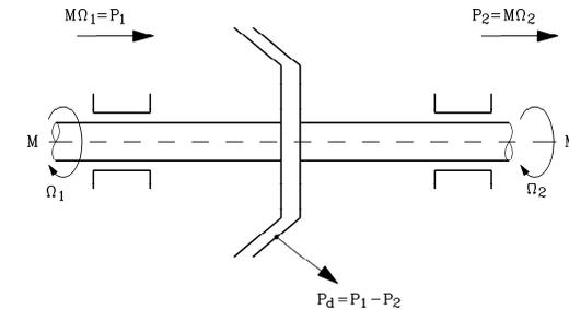
Fig. 5.11: A slip clutch is a mechanical analogy for an induction machine
