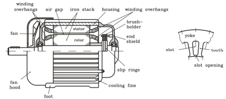
Fig. 5.1: Longitudinal cross-section of a fan-cooled slipring induction motor and detailed drawing of the stator lamination with slots for the winding
