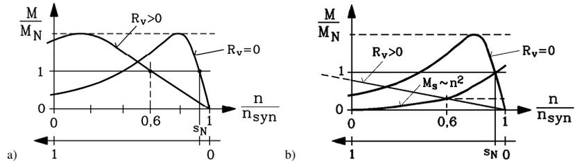
Fig. 5.18:  $M(n)$ -characteristic of a slipring-induction motor with external resistances as variable speed drive a) constant load torque, b) load torque increases with the square of the motor speed (pump, variable flow rate)
