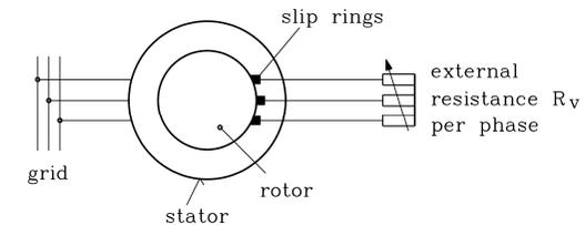
**Fig. 5.16:** Using external resistances via sliprings in the rotor circuit of an induction machine
