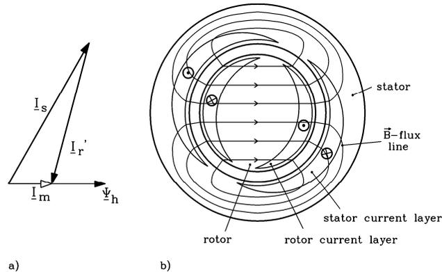
Fig. 5.6: Rated operating point of an induction machine:
