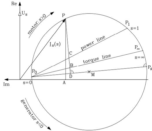
Fig. 5.13: Circle diagram of an induction machine at  $R_s > 0$  (OSSANNA's circle)
