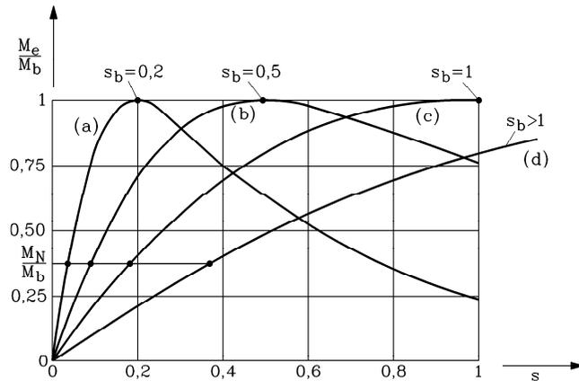
Fig. 5.17: Torque characteristic of a slipping-induction motor ( $M_b/M_N = 2.65$ ) with additional rotor resistances. Without external resistances (a), the breakdown torque occurs at the slip 0.2, the starting torque is as small as  $0.24M_b$ . However, with use of an external resistance per phase  $R_v = 4R_r$ , we get “starting torque” = “breakdown torque” (c).
