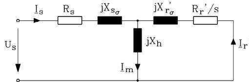
Fig. 5.5: T-equivalent circuit per phase for the field fundamental of an induction machine for currents and voltages changing sinusoidally with time (iron losses  $P_{Fe}$  neglected,  $U_s$  assumed as real)
