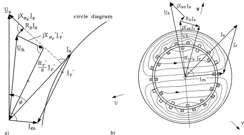
Fig. 5.7: Typical phasor diagram per phase of an induction machine: rated operating point, rated slip.
