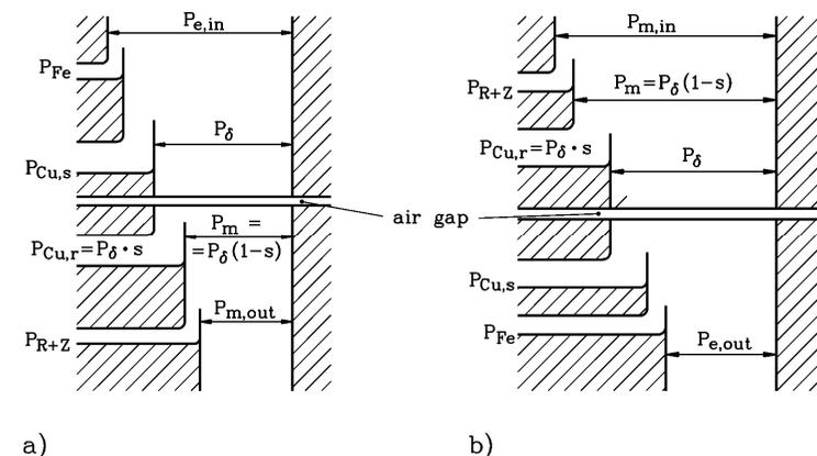
Fig. 5.10: Power flow in an induction machine a) motor operation, b) generator operation
