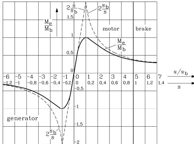
Fig. 5.9: Electromagnetic torque of an induction machine depending on the slip, stator resistance  $R_s = 0$  (KLOSS' formula), at the example of breakdown slip  $s_b = 0.2$ .
