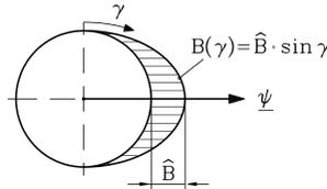
Fig. 5.3: In the air gap, the fundamental field is sinusoidally distributed along the circumference and can be represented by a “space vector”  $\underline{\mathcal{B}}$
