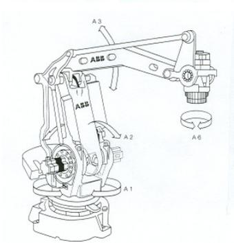
Fig. 9.22: One-arm-robot with permanent magnet synchronous machines used as drives
