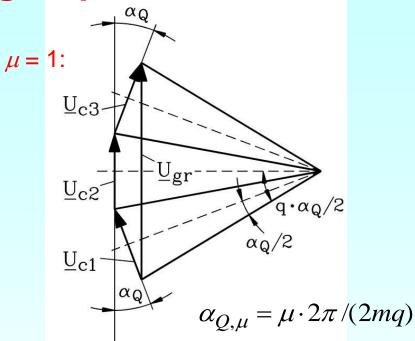
•The induced sinusoidal AC voltage per coil group is the sum of complex phasors of the q coils. The coil voltage phasors are phase shifted by angle  $\alpha_{Q,\mu}$  between adjacent coils:
