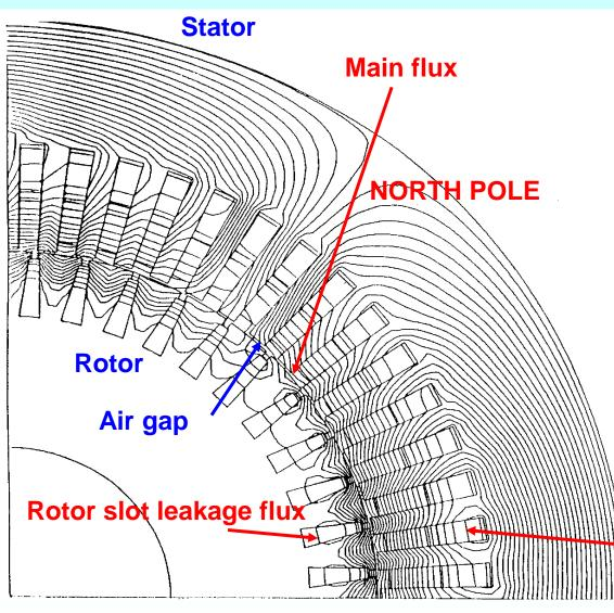
Main flux: Links stator and rotor winding; field lines cross the air gap
