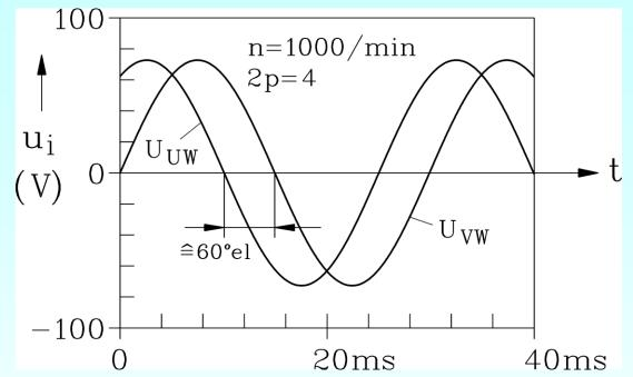
Measured no-load voltage line-to-line of a 4 pole PM synchronous generator at 1000/min, q = 3, skewed slots, star connection, **showing nearly ideal sine wave back EMF** *Fourier*-Analysis of no-load voltage:  $\mu = 1$ : 33.5 Hz, 74.8 V
