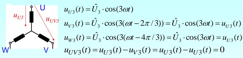
If the stator winding is star connected, the third harmonic voltages in all three phases U, V, W are IN phase and IDENTICAL !
