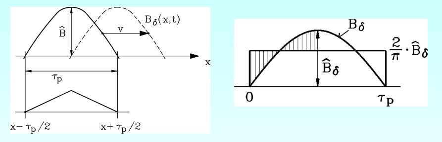
• Sinusoidal moving wave  $B_{\delta 1}(x,t) = \hat{B}_{\delta 1} \cos(x\pi/\tau_p - \omega t)$  causes changing coil flux  $\Phi(t)$  $\Phi(t) = l \int_{-\tau_p/2}^{\tau_p/2} B_{\delta 1}(x,t) dx = \frac{2}{\pi} \tau_p l \hat{B}_{\delta 1} \cdot \cos \omega t \implies \text{flux linkage } \Psi(t) = N_c \Phi(t)$
