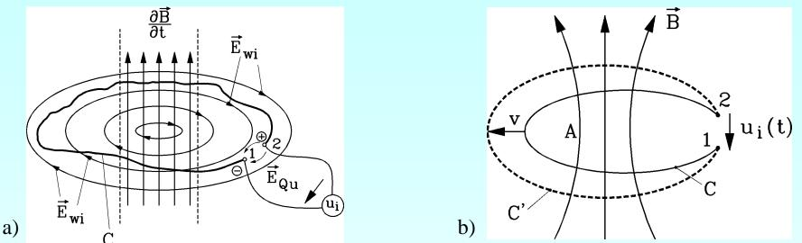
Each change of flux  $\Phi$ , which is linked to conductor loop *C*, causes an induced voltage  $u_i$  in that loop; the induced voltage is the negative rate of change of the linked flux.  $u_i = -d\Phi/dt$  Fluß:  $\Phi = \int \vec{B} \cdot d\vec{A}$
