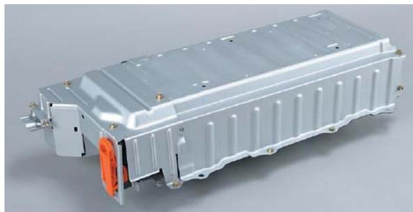
Fig. 6.2-2: NiMH-Battery by Toyota (Toyota Hybrid System THS II, press information, [www.toyota.co.jp](http://www.toyota.co.jp), 2003)
