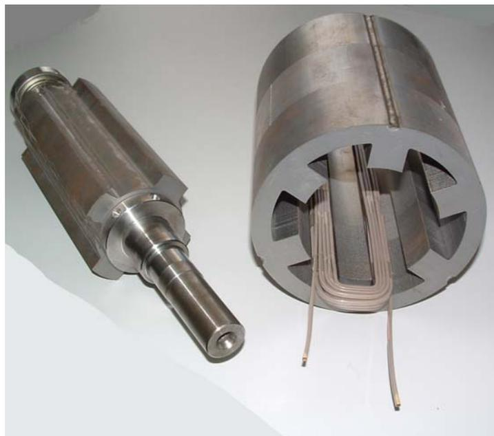
Fig. 4.1.4-6: Rotor and stator stack of a 3-phase, two-pole 6/4-switched reluctance motor
