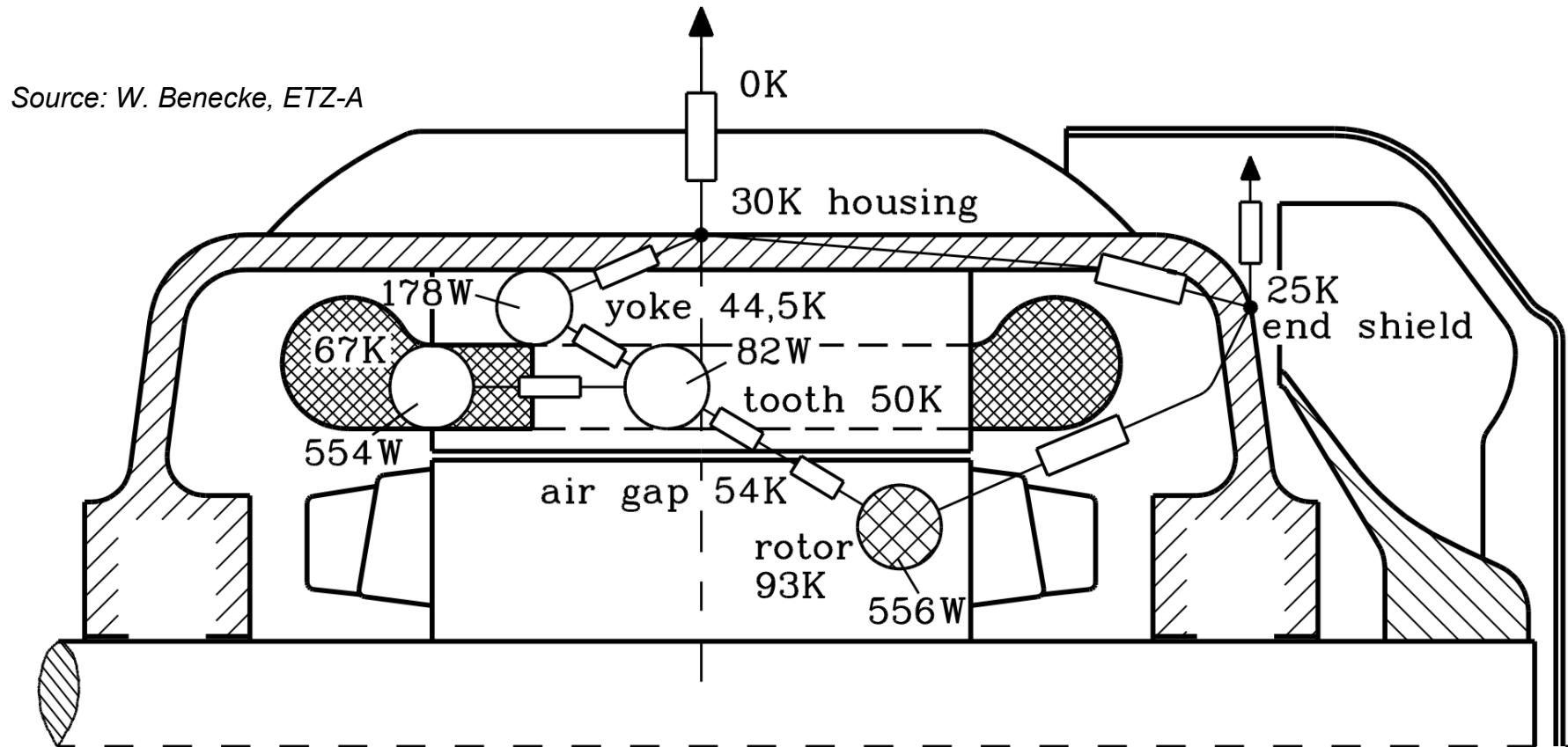
Example: Totally enclosed cage induction machine with shaft mounted fan, 11 kW, 4-pole, 50 Hz, 1450/min rated speed, Thermal Class B
