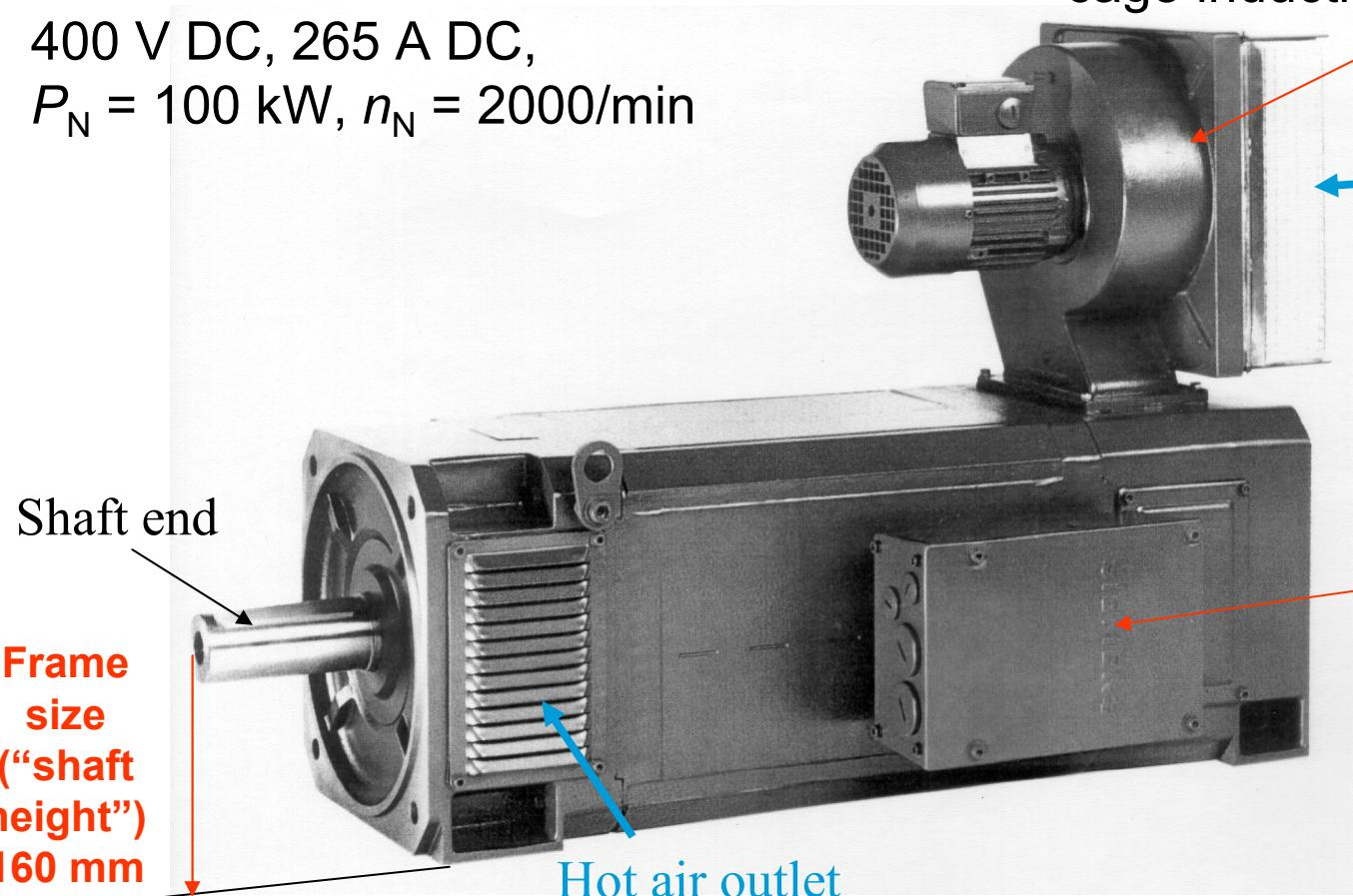
Radial fan, driven by extra 2-pole cage induction motor (IC41)
