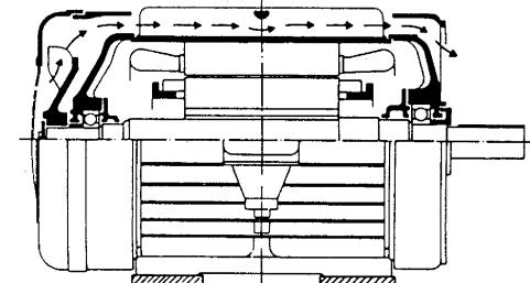
Thermal Class F:  $40^{\circ}\text{C} + 105 \text{ K} + 10 \text{ K} = 155^{\circ}\text{C}$  (rated power  $\leq 5 \text{ MW}$ )
