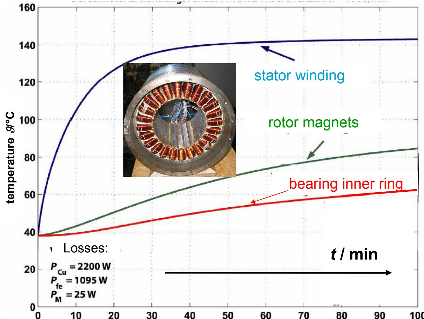
16-pole PM synchronous motor,
