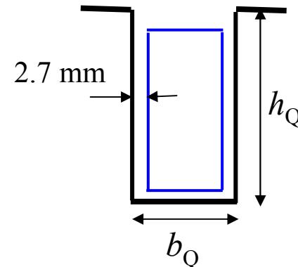
Thermal conductivity resistance from copper to iron:
