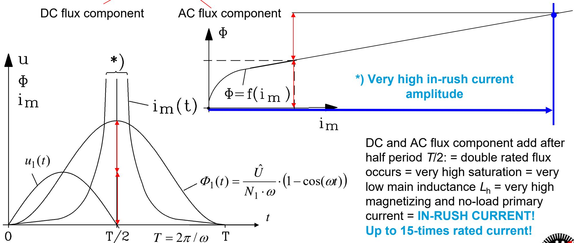
DC and AC flux component add after half period  $T/2$ : = double rated flux occurs = very high saturation = very low main inductance  $L_h$  = very high magnetizing and no-load primary current = **IN-RUSH CURRENT!**
