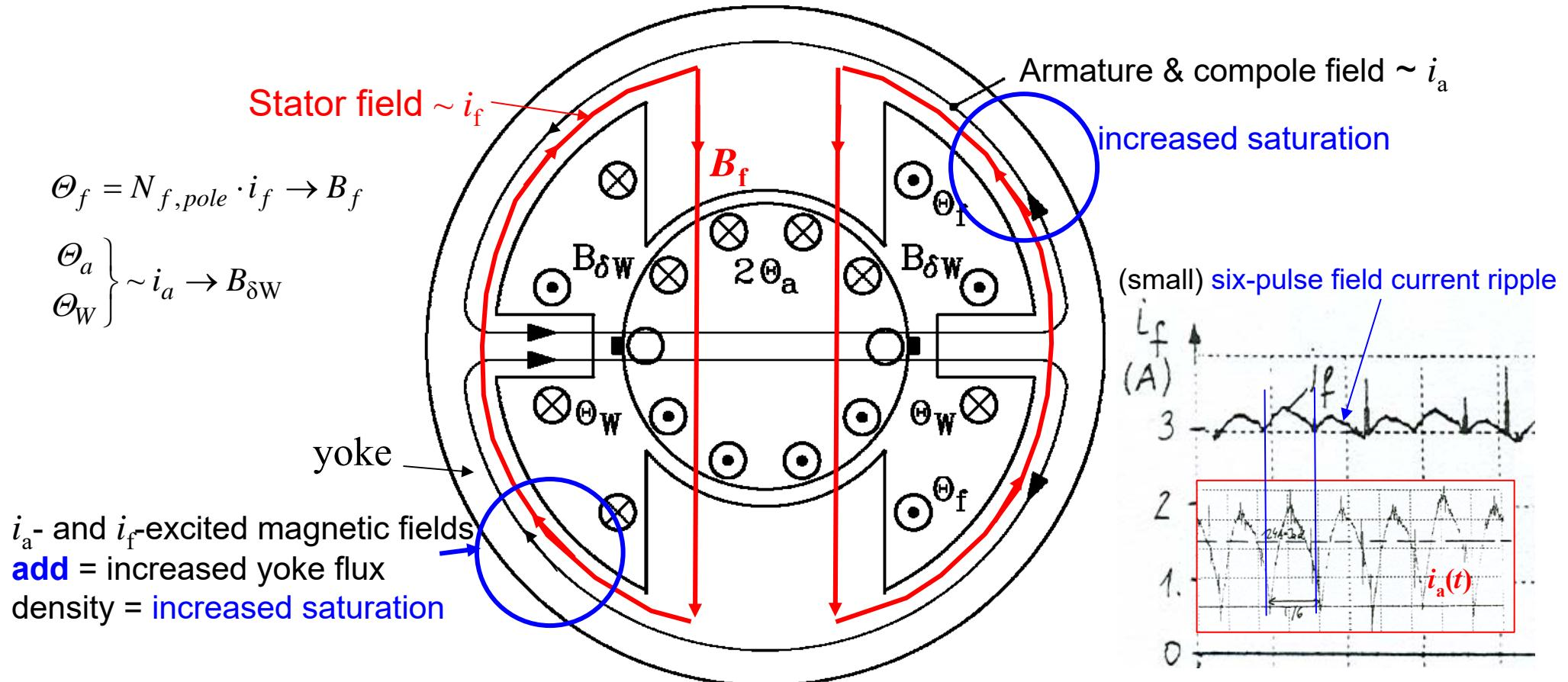
Due to the magnetic **common path** in the yoke a change of the armature current  $i_a$  causes a change of yoke iron permeability  $\mu_{Fe}$ . Hence also the stator field  $B_f$  changes and induces a voltages in the field coil, which causes a (small) **six-pulse ripple of field current  $i_f$** .
