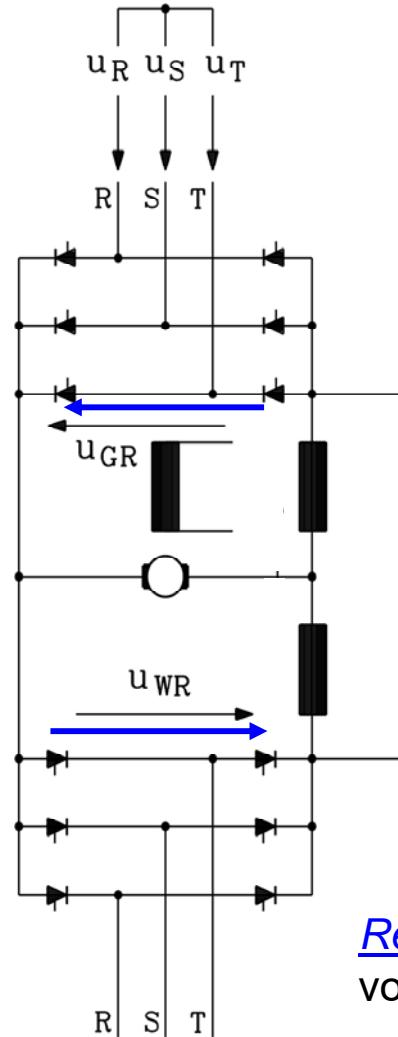
Two anti-parallel bridges operate with the same average output voltage in parallel.
