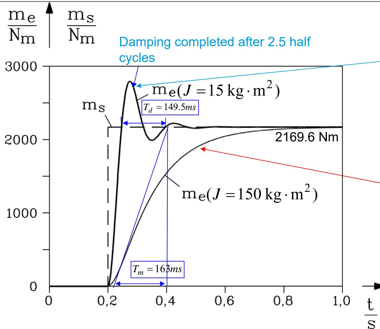
At **low total inertia** DC machine is oscillating
