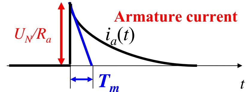
**Attention:** Starting resistor is necessary:
