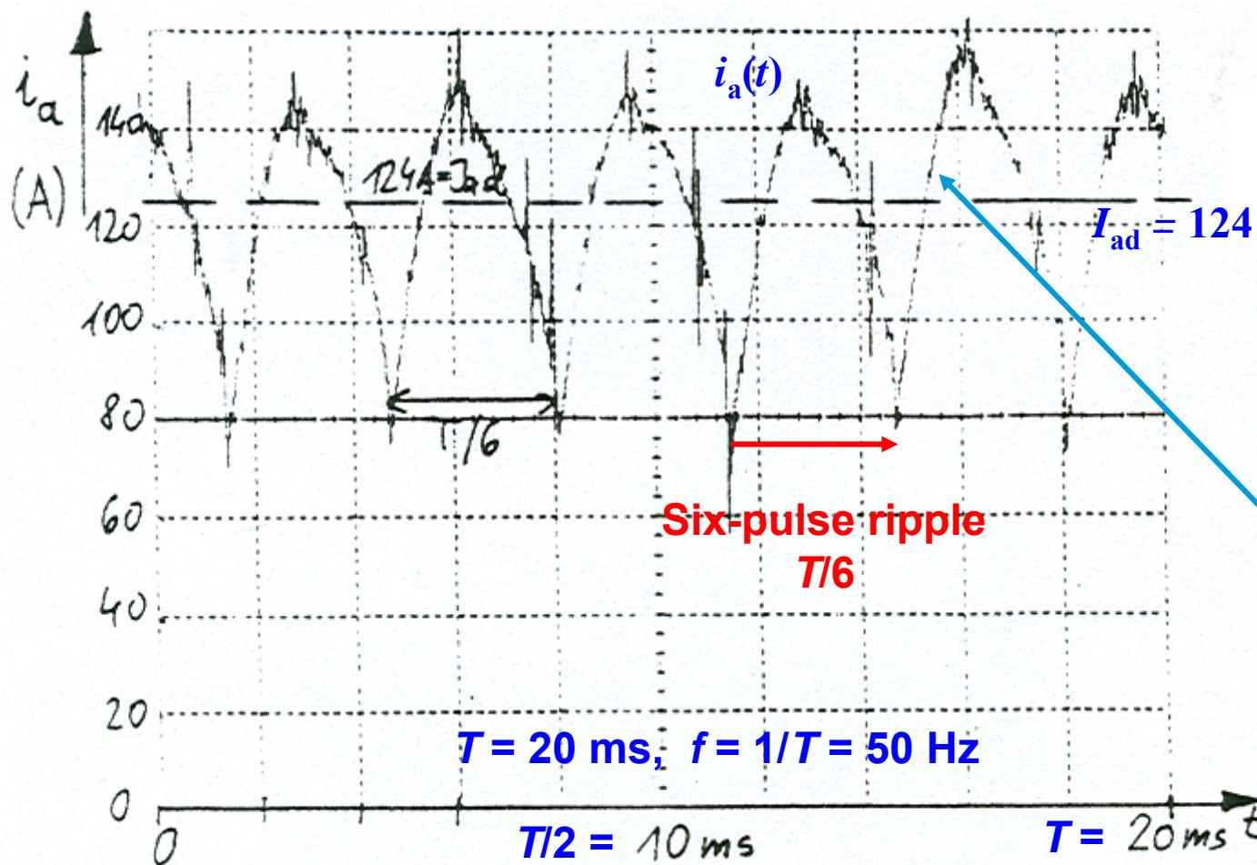
Measured armature current
