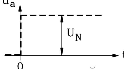
$$\frac{d^2 i_a}{dt^2} + \frac{1}{T_a} \cdot \frac{di_a}{dt} + \frac{1}{T_a \cdot T_m} \cdot i_a = \frac{1}{T_a \cdot R_a} \cdot \frac{du_a}{dt} + \frac{1}{T_a \cdot T_m} \cdot \frac{1}{k_2 \Phi} \cdot m_s$$
