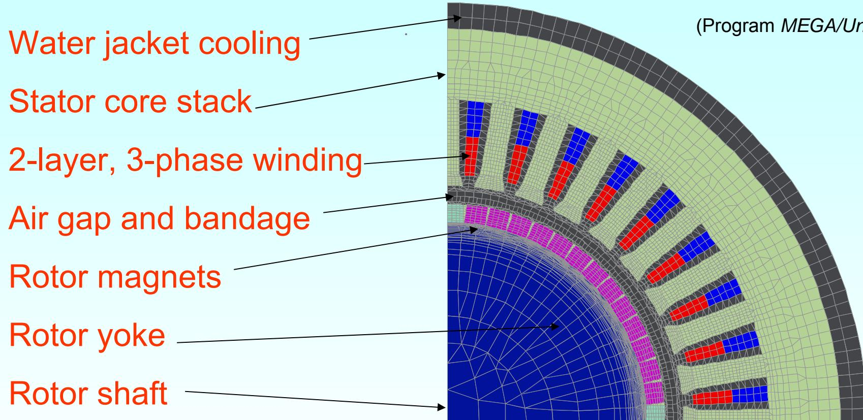
Results: solid rotor yoke: too high losses with block-voltage supply
