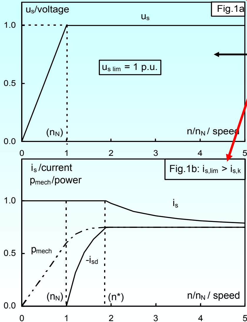
a) Voltage characteristic of inverter with voltage limit
