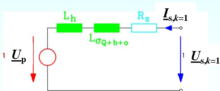
Equivalent circuit of the PM synchronous machine for a harmonic frequency  $k \cdot f_s$
