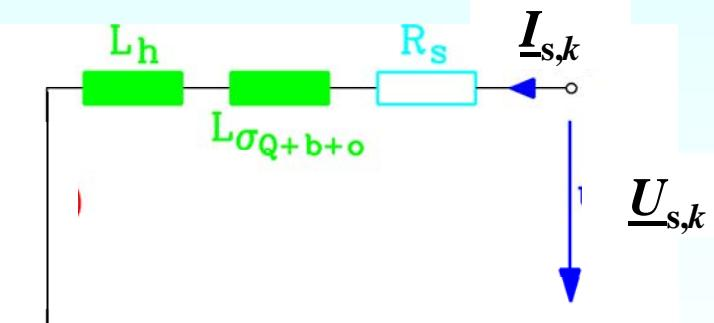
$$\underline{I}_{s,k} \approx \frac{\underline{U}_{s,k}}{\sqrt{R_s^2 + (k\omega_s)^2 \cdot (L_{s\sigma} + L_h)^2}}$$
