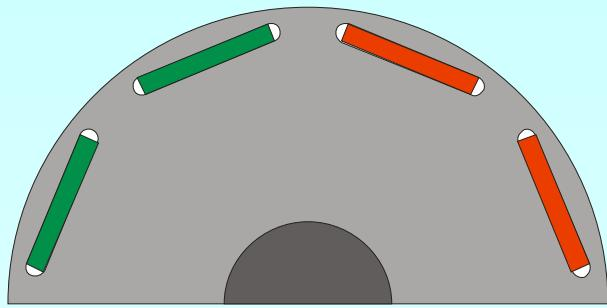
Magnets are fixed by rotors sheet:
