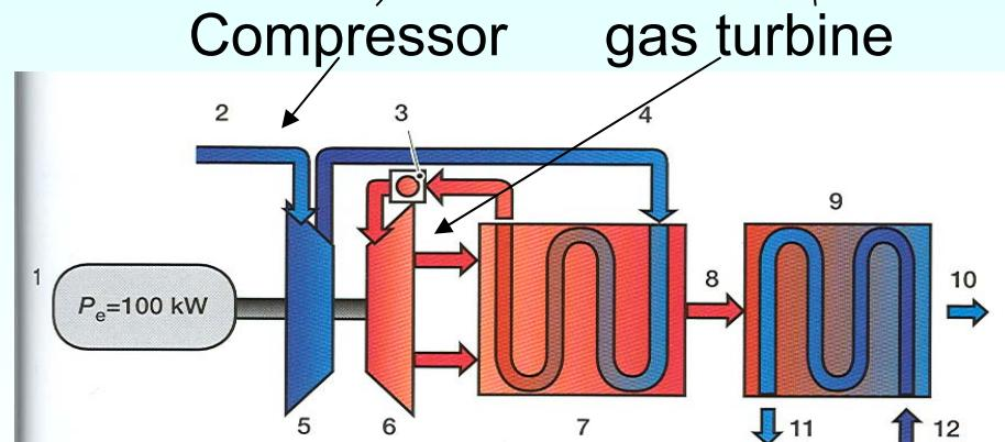
„Micro“-gas turbine: Advantage: Co-generation of heat and electricity, high thermal efficiency - **high utilization of gas energy**
