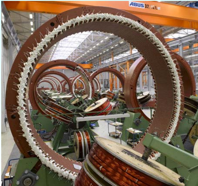
Integer-slot q = 1 round wire low voltage single layer stator 3-phase winding manufacturing
