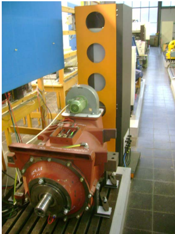
Test bench for measurements of CM currents at a 240 kW induction motor
