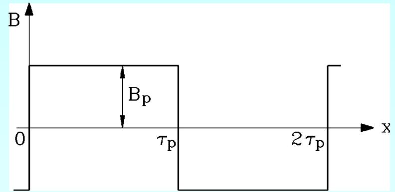
PM rotor with surface mounted magnets
