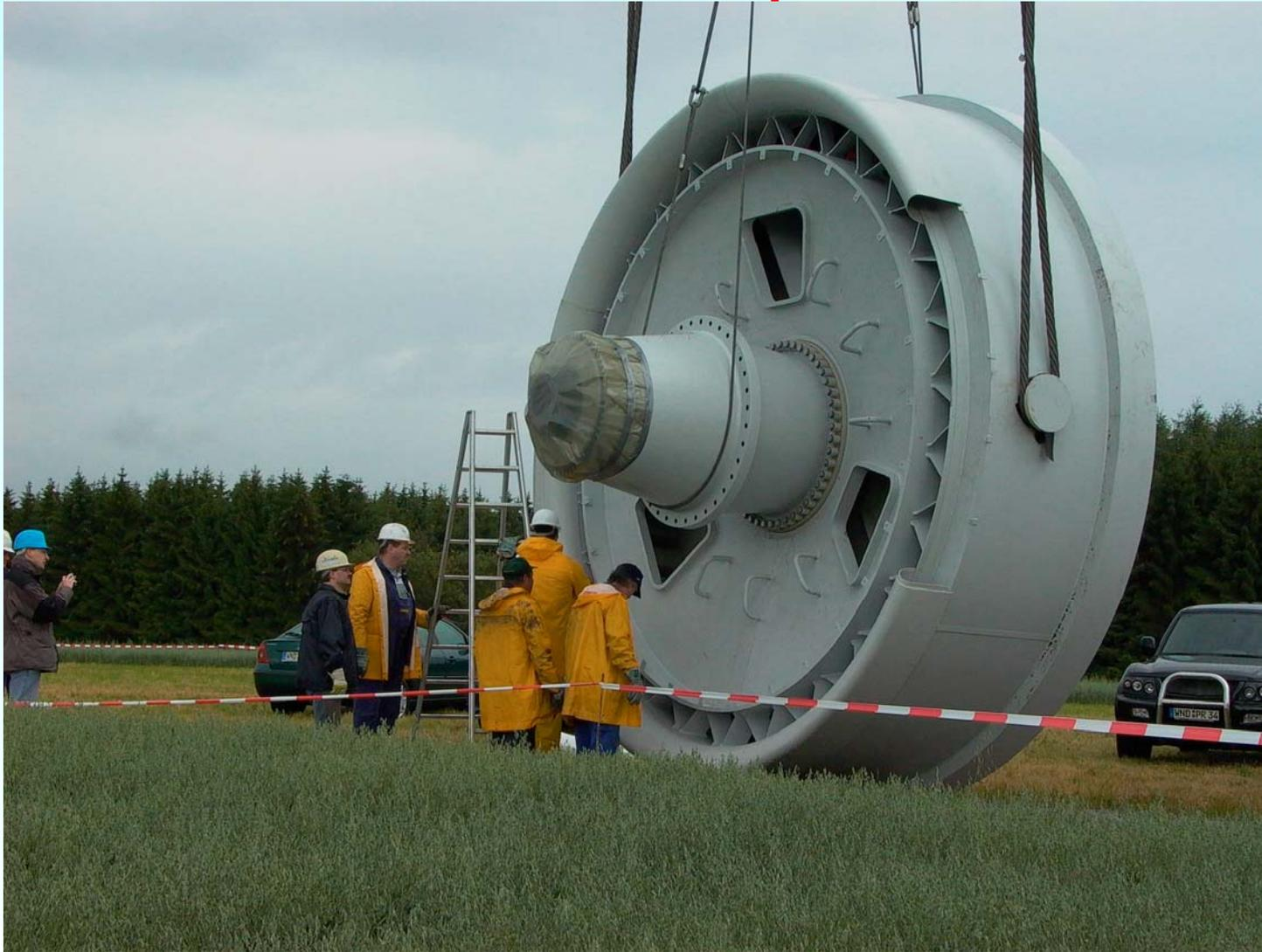
Outer PM rotor to increase torque by increased bore diameter
