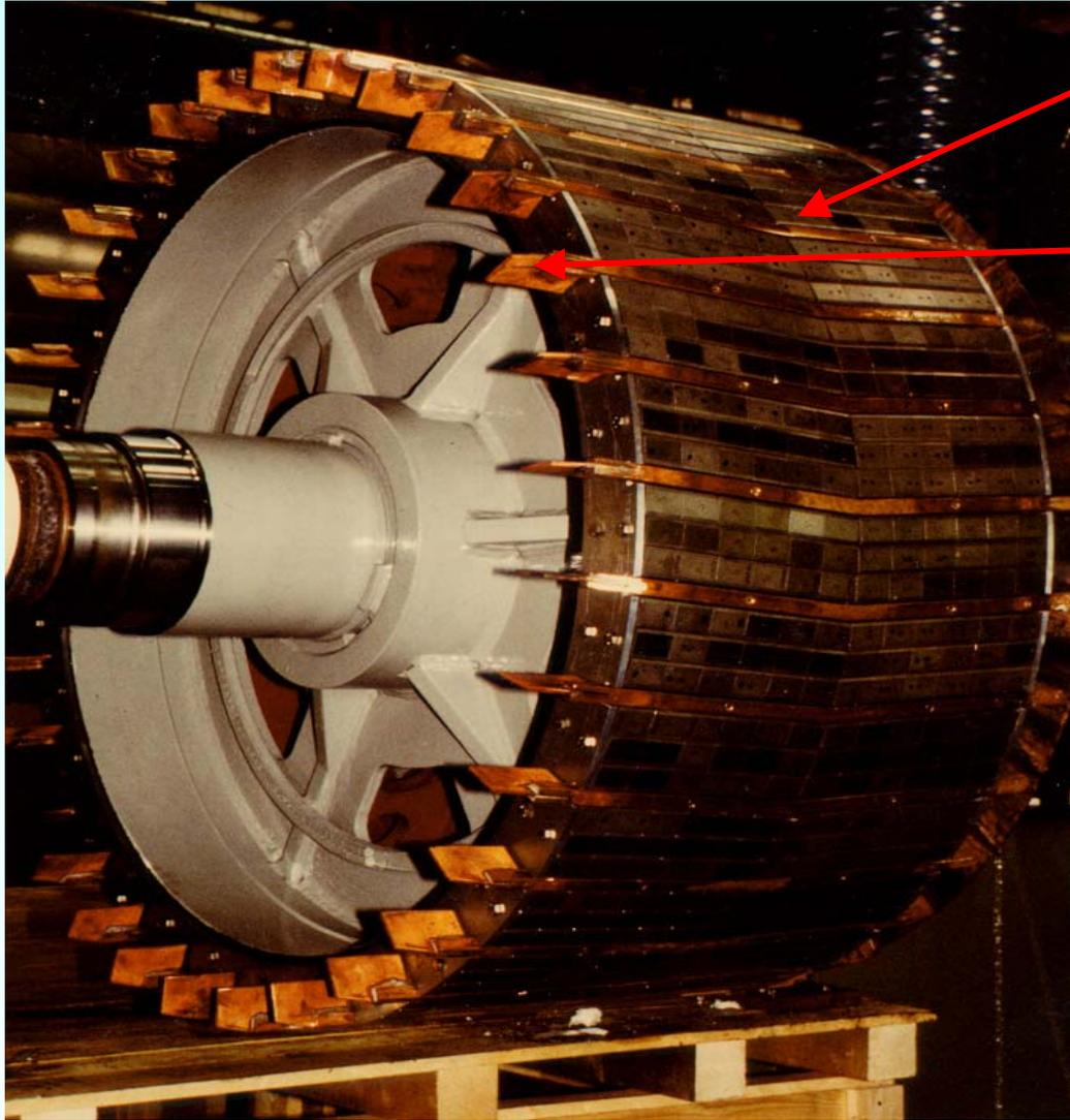
Skewed rotor magnets to reduce cogging torque
