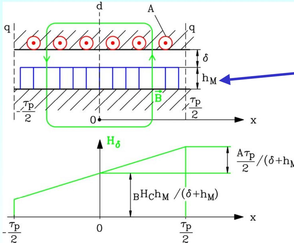
**Surface mounted magnets, glued to rotor**
