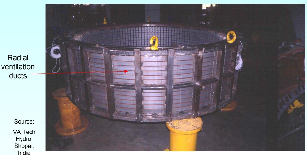
Low speed operating synchronous generator, river power plant
