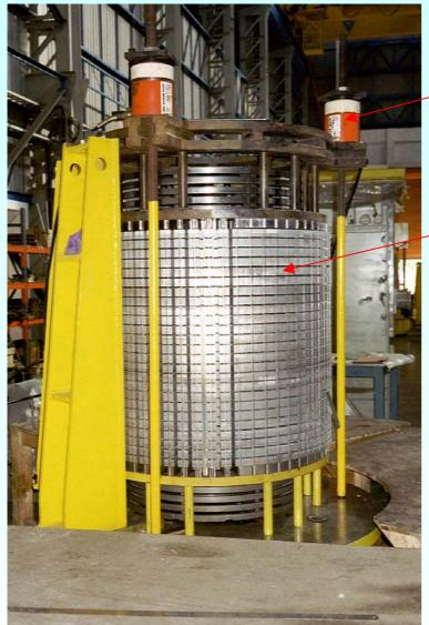
Hydraulic cylinders for pressing rotor iron stack
