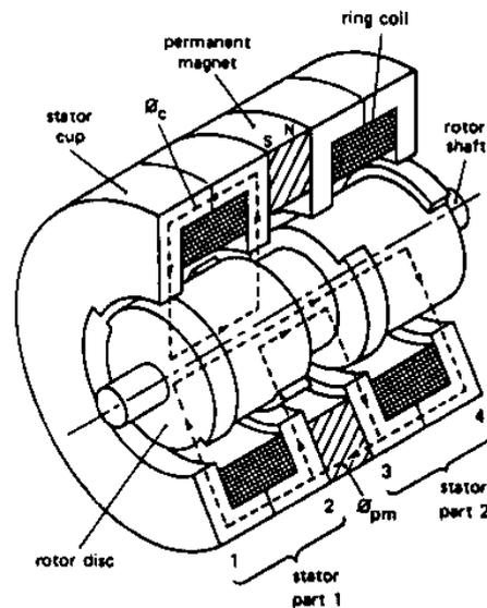
Fig. 8.2.2-1: 2-phase hybrid stepper motors with homo-polar flux arrangement and bipolar current operation: a) Permanent magnet in the rotor, 3 rotor teeth per half machine, 4 stator teeth (Stölting *et al.*, *El. Kleinmaschinen*, Teubner, 1987), b) Permanent magnet in the stator, claw pole stator, 1 tooth in stator and rotor per radial plane:  $\Phi_c$ : coil flux,  $\Phi_{PM}$ : PM flux (Philips Comp.)
