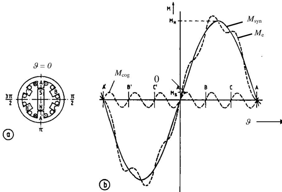
Fig. 8.4.1-1: Three-phase, 2-pole PM-stepper motor ( $m = 3, 2p = 2$ ): a) cross section: Rotor S-pole at position A, load angle is zero, b) static torque for increasing/decreasing load angle. For the cogging torque six periods with the positions A, B, C, A', B', C' exist. (Stölting et al., *El. Kleinmaschinen*, Teubner, 1987)
