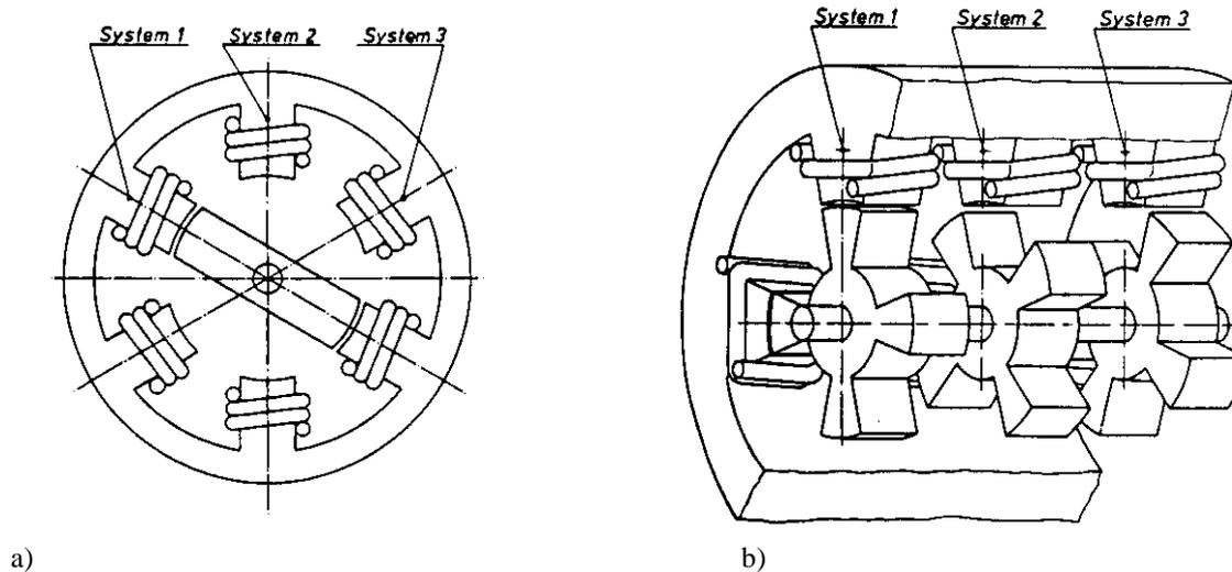
Fig. 8.1-1: Design examples of the multi-phase stator winding of a VR-motor with  $m$  phases and  $Q_r$  rotor teeth
