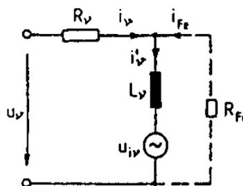
Fig. 8.3-2: Electrical equivalent circuit of the  $v^{\text{th}}$  stator phase ( $R_v$ ,  $L_v$ : phase resistance and inductance,  $u_{iv}$ : back EMF per phase,  $R_{fe}$ : equivalent resistance for considering the iron losses per phase) (Stöling et al., *El. Kleinmaschinen*, Teubner, 1987)
