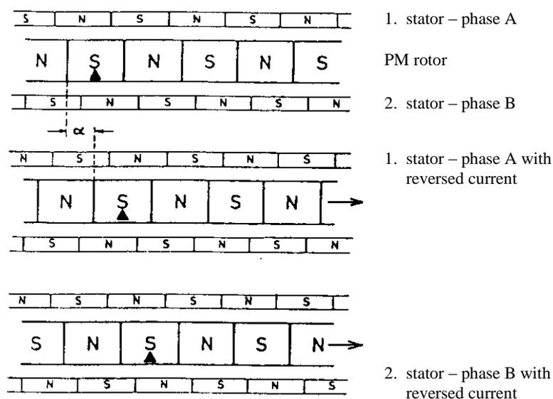
Fig. 8.2.1-2: Current feeding sequence of a two-phase claw pole PM stepper motor
