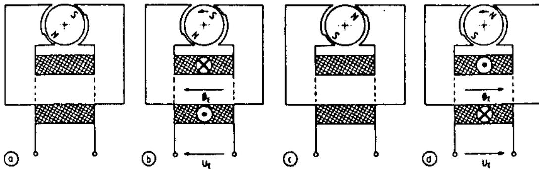
Fig. 8.2.3-1: Single phase PM stepper motor with asymmetric poles by narrower air gap at one pole side (Stölting et al., El. Kleinmaschinen, Teubner, 1987)
