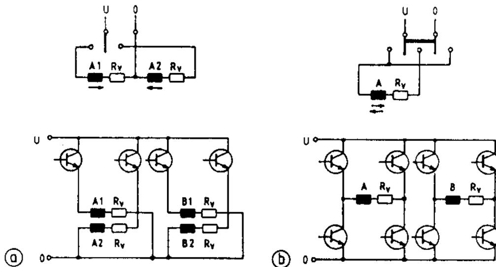
Fig. 8.3-1: Driving circuits for stepper motors with a) uni-polar, b) bipolar current. Free-wheeling diodes are omitted here for clarity. The resistance  $R_v$  are used to reduce the electric time constant (Stölting et al., El. Kleinmaschinen, Teubner, 1987)
