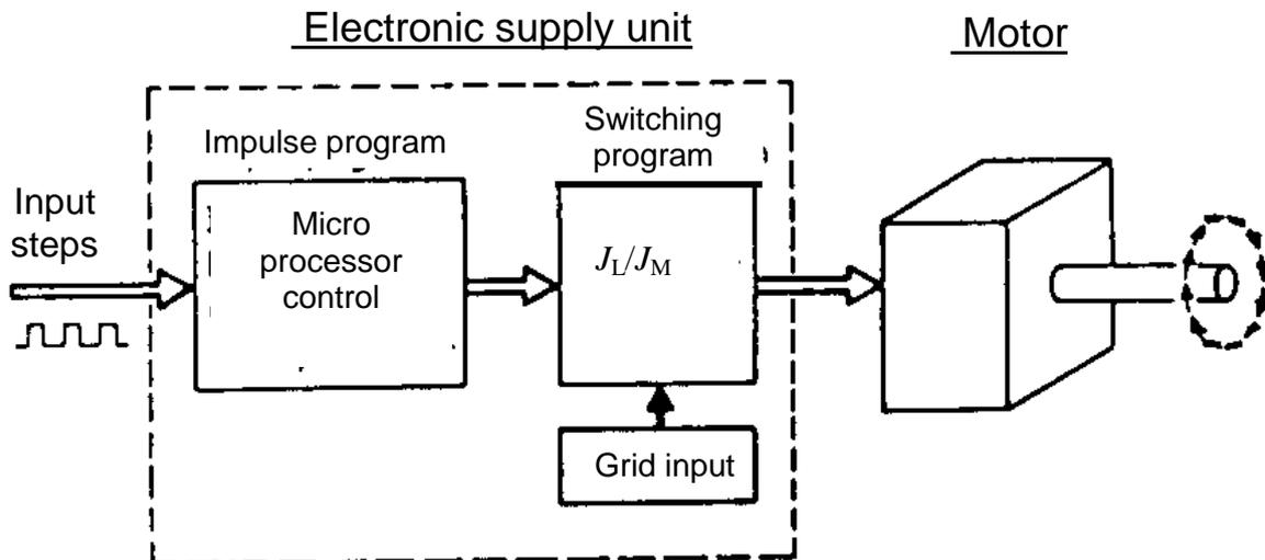
Fig. 8-1: Basic scheme of a stepper drive (Stölting et al., El. Kleinmaschinen, Teubner, 1987)
