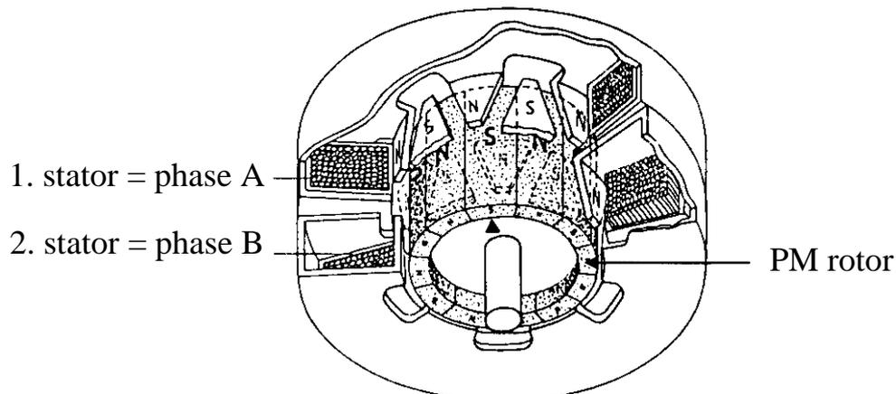
Fig. 8.2.1-1: PM-claw pole stepper motor,  $m = 2$ ,  $2p = 12$  (Stölting et al., *El. Kleinmaschinen*, Teubner, 1987)
