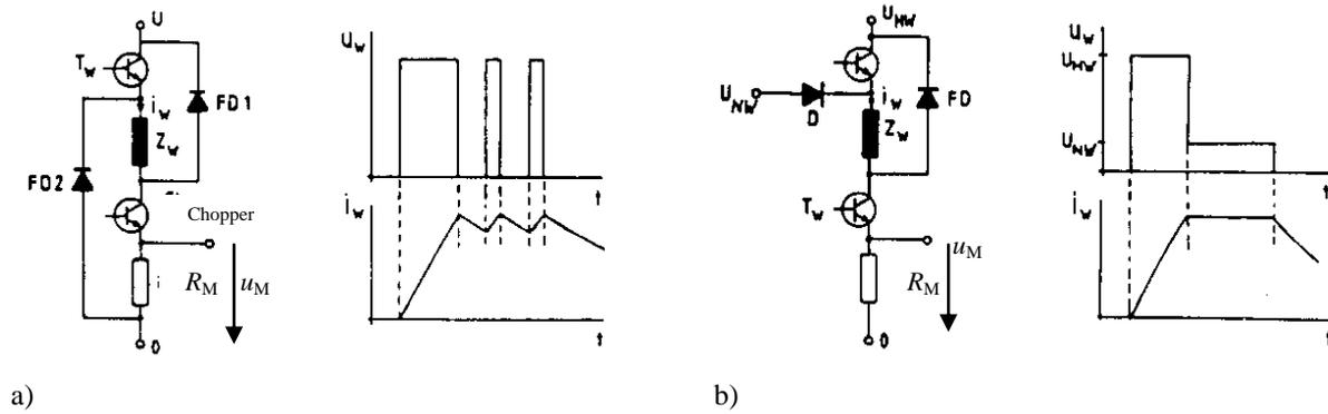
Fig. 8.3-3: Driving circuits for stepper motors (winding impedance  $Z_w$ ) (Stölting et al., *El. Kleinmaschinen, Teubner*, 1987)
