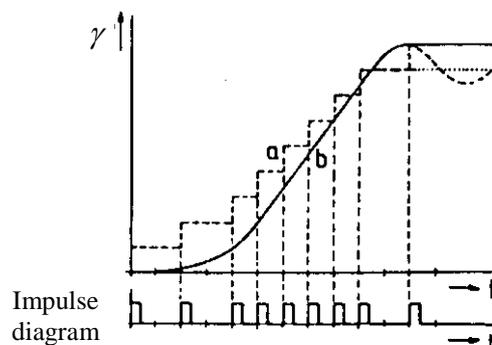
Fig. 8.3-4: Delayed last step: According to the current impulses (below) the wanted rotor position (dashed line a), expressed as rotational angle  $\gamma$ , is followed by the real motion (solid line b). At the maximum overshoot of step  $N-1$  the last current impulse is commanded, hence avoiding the overshoot at step  $N$  (Stölting et al., *El. Kleinmaschinen, Teubner*, 1987).
