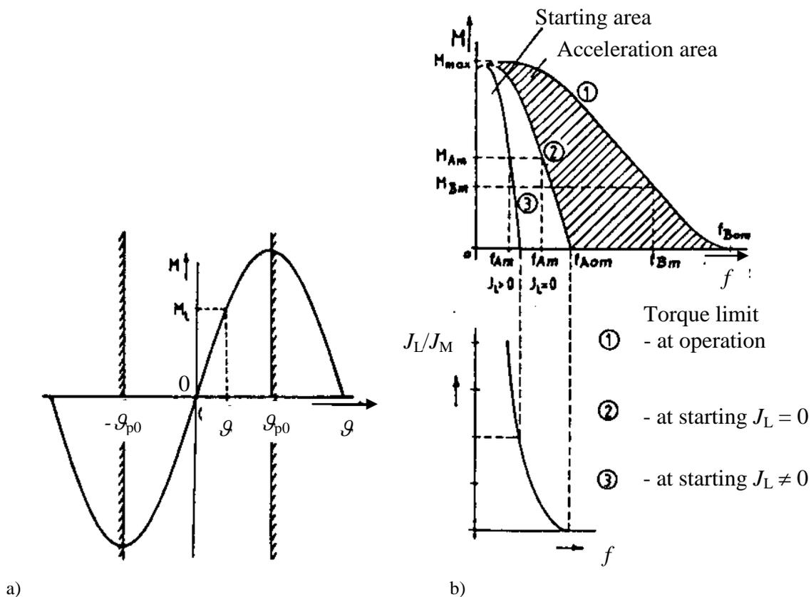
Fig. 8.4.1-2: a) Static load angle  $g$  of a stepper motor, that is loaded at the shaft with a torque  $M_s$ , b) dynamic torque characteristic of a stepper motor in dependence of the stepping frequency  $f$ : 1: Torque limit at operation with constant  $f$ , 2: Torque limit at no-load starting (no load coupled:  $J_L = 0$ ), 3: as 2, but with coupled load inertia  $J_L > 0$  ( $J_L, J_M$ : Load and motor rotor inertia)
